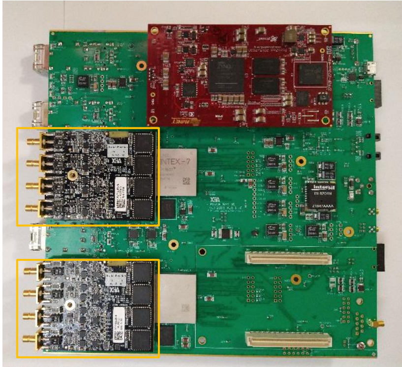
Main board with ADC daughtercards (black) and Zynq controller module (red).
