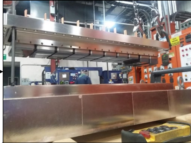
Lowering tile/backer flange assembly into housing
