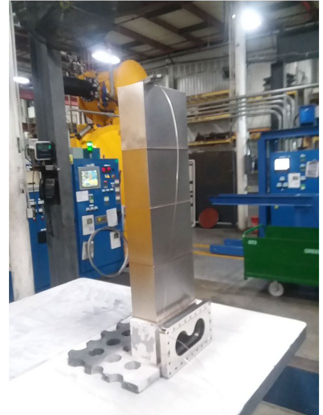
Parts stacked with braze alloy - thermocouples applied, ready for intermediate braze step
