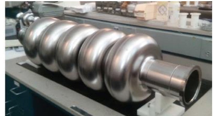
800 MHz cavity built at JLAB for PERLE prototype
