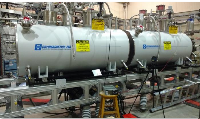
Electron beam ion source EBIS with polarized ^3\text{He} extension
