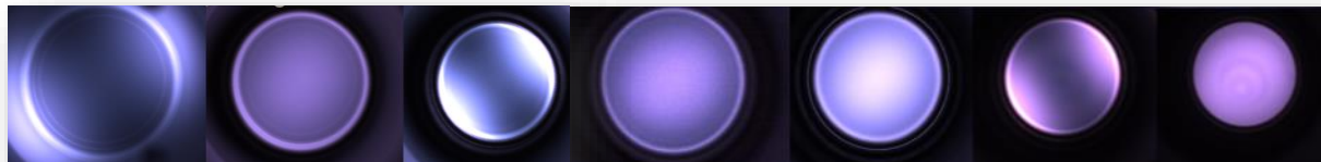
Plasma established in all 7 cells of a C100 cavity.
