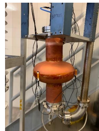
RDT-10 1.3 GHz Nb 3 Sn cavity
