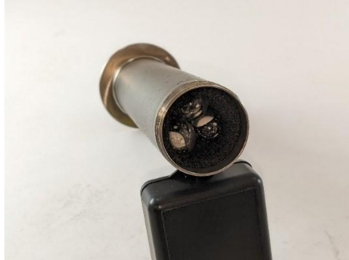
3 Ampoules Loaded into the Titanium Rabbit for Irradiation
