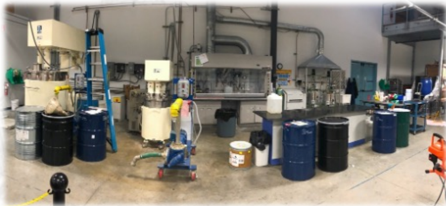
250-gal, 55-gal, 1-10 L in hood, two 20L, and one 100 L reactor
