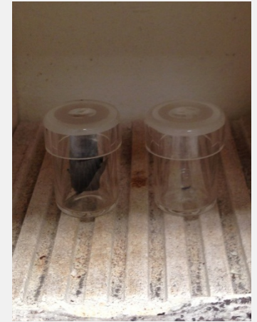
Samples (with crucible covers) in muffle furnace before heating
