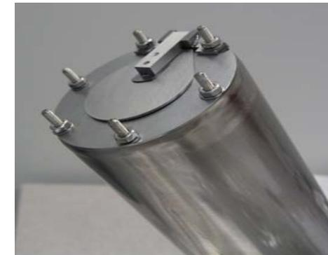
Photo of the output end of the independently cooled shroud/shutter assembly for phosphorus flux abatement. The shutter can change states in a sub-second time scale.
