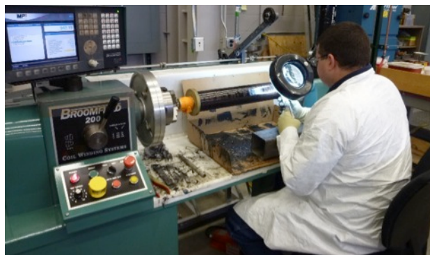
Superconducting magnet fabrication
