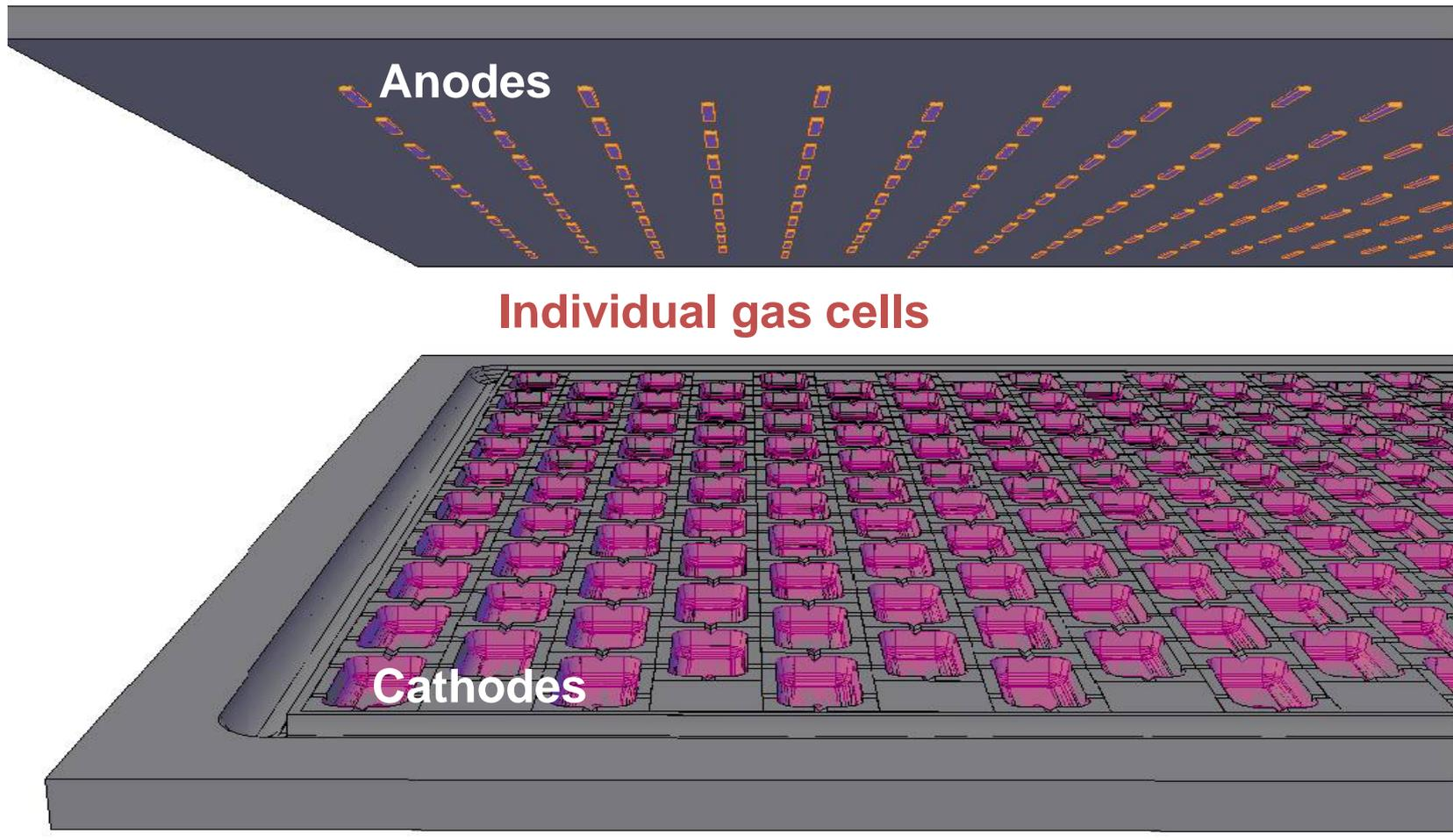
Perspective view of a pixel array with gas channels. Metallized cathode cavities on bottom plate with *vias* to HV bus. Anodes on top plate.
