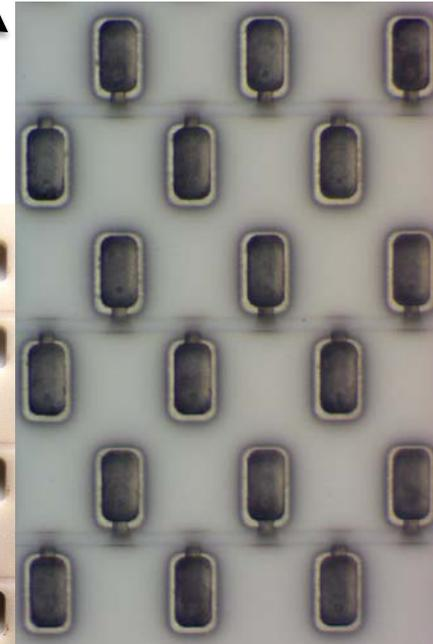
Bottom Side – quench resistor for each pixel.
