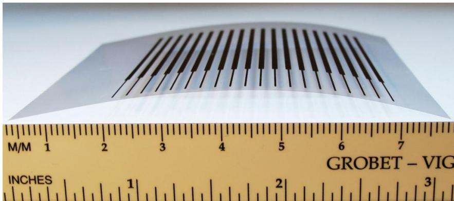
Top Row: Photos of **0.026, 0.20 & 0.30 mm** thick glass. Electrode pitch is **2.54 mm**.
