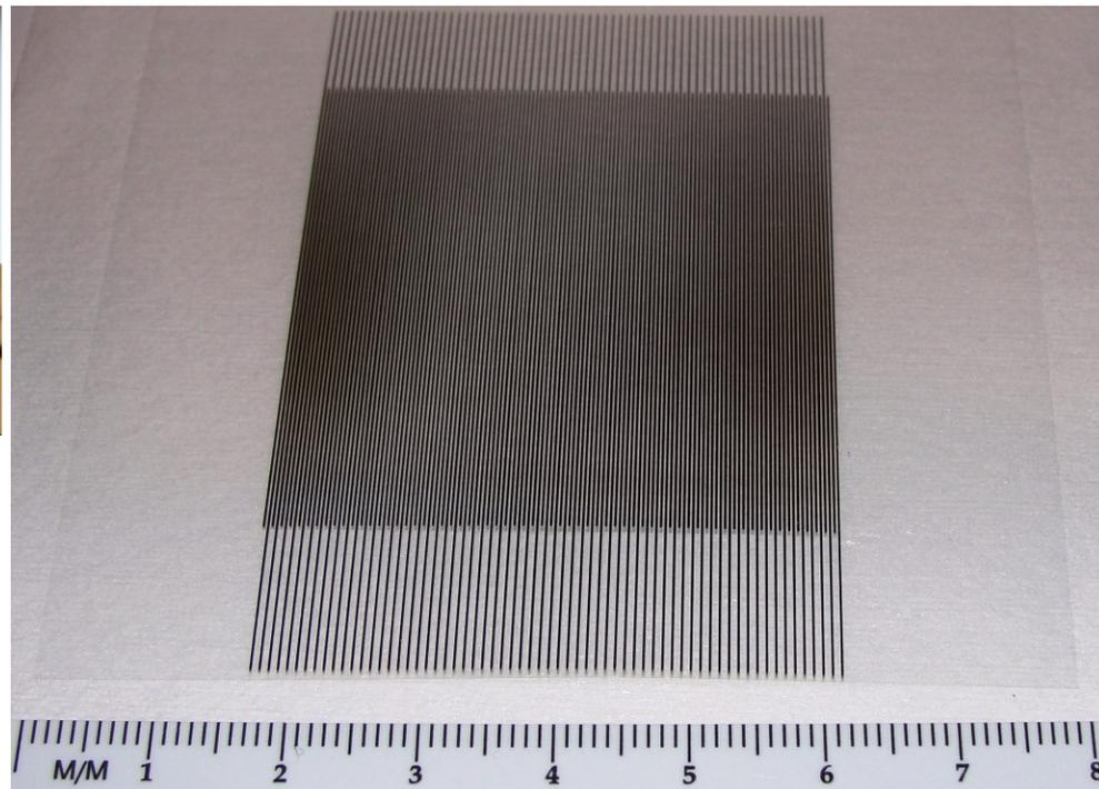
Bottom Right: High resolution electrodes on 26  $\mu\text{m}$  thick glass. Electrode pitch in active area (center) is **0.35 mm**, electrode width is 0.15 mm. The narrow electrode width & spacing on the slightly bowed glass created the Lissajou type interference pattern, which is an optical artifact of image magnification and viewing angle. The actual electrode pattern is very uniform.
