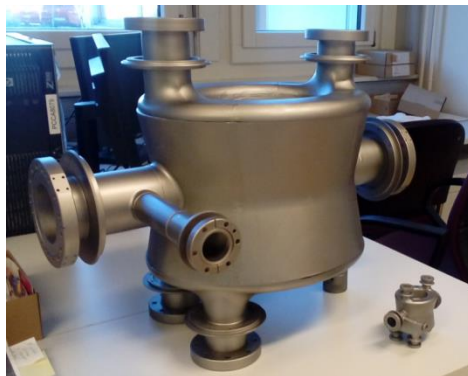
3D printed Double Quarter Wave Crab Cavity at CERN (Resin with coating).
