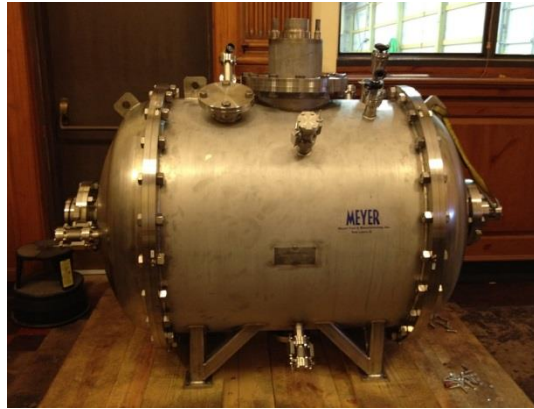
112 MHz SRF electron gun cavity for CeC
