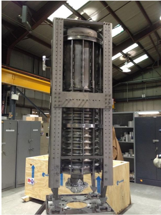
56 MHz SRF cavity for increasing RHIC luminosity
