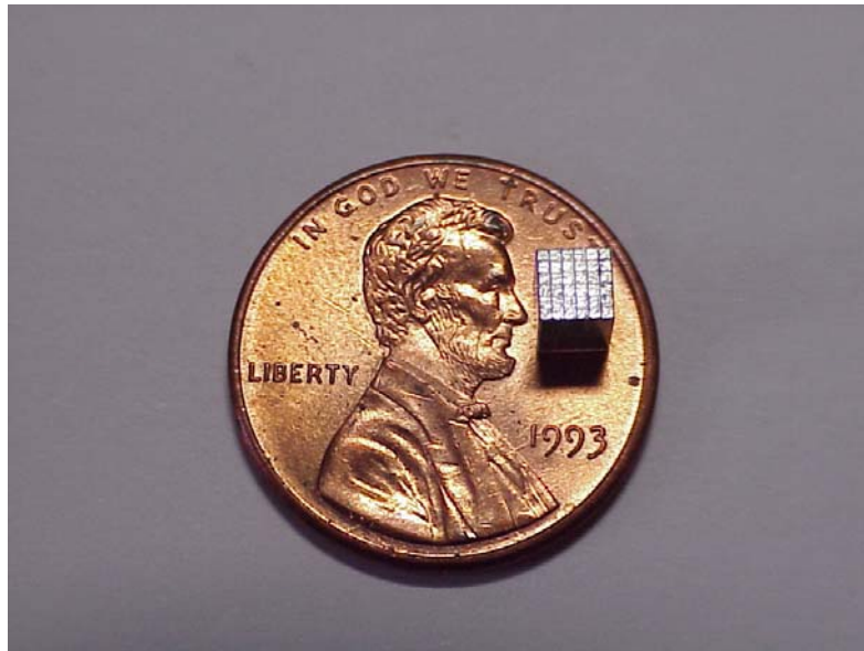
6 x 6 LYSO array having 500 \mu\text{m} pixels
