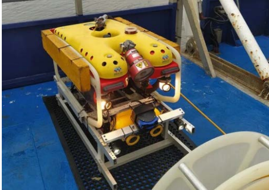
Figure 10: Underwater Drone for Wind Farm Foundation Inspections
