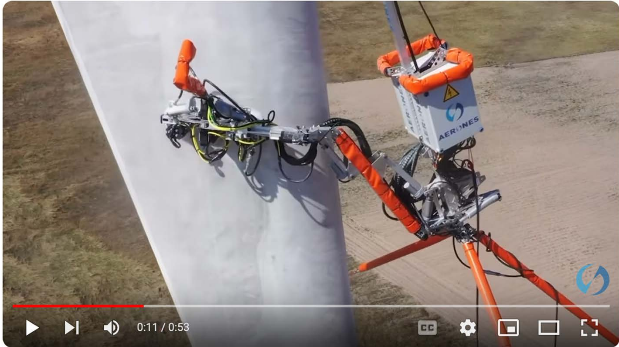
Figure 14: Aeronex Robotic Wind Turbine Blade & Tower Cleaning
