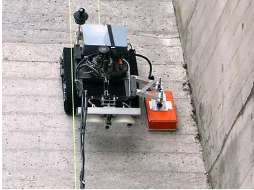
Figure 12: International Climbing Machine – Suction Held Robot Source: International Climbing Machines, 2023 57
