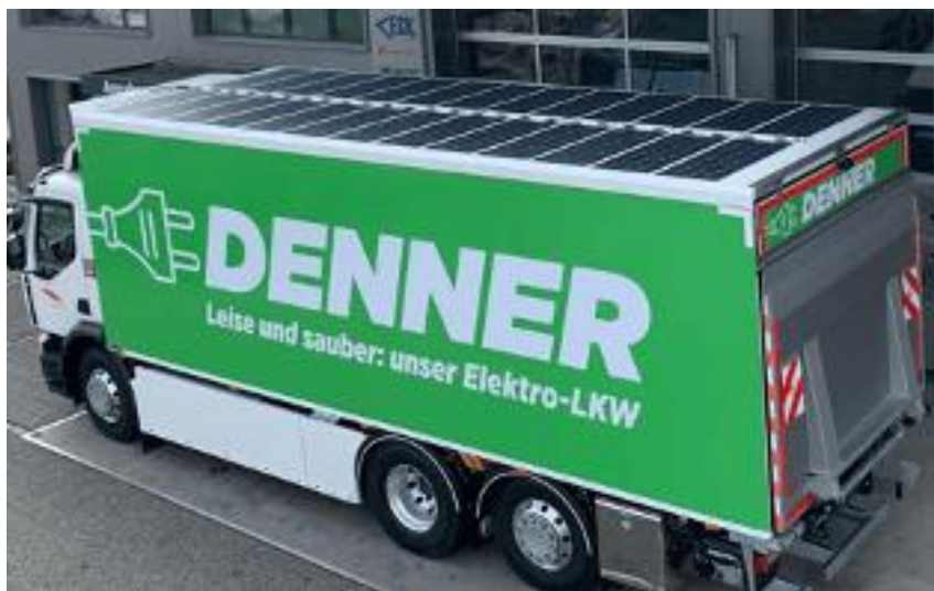
Figure 30: Rhyner Logistik truck outfitted solar panels on rooftop
