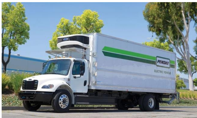
Figure 32: Class-7 Freightliner eM2 Battery-electric Truck with Carrier Transicold's Supra e11 eCool Electric Refrigeration
