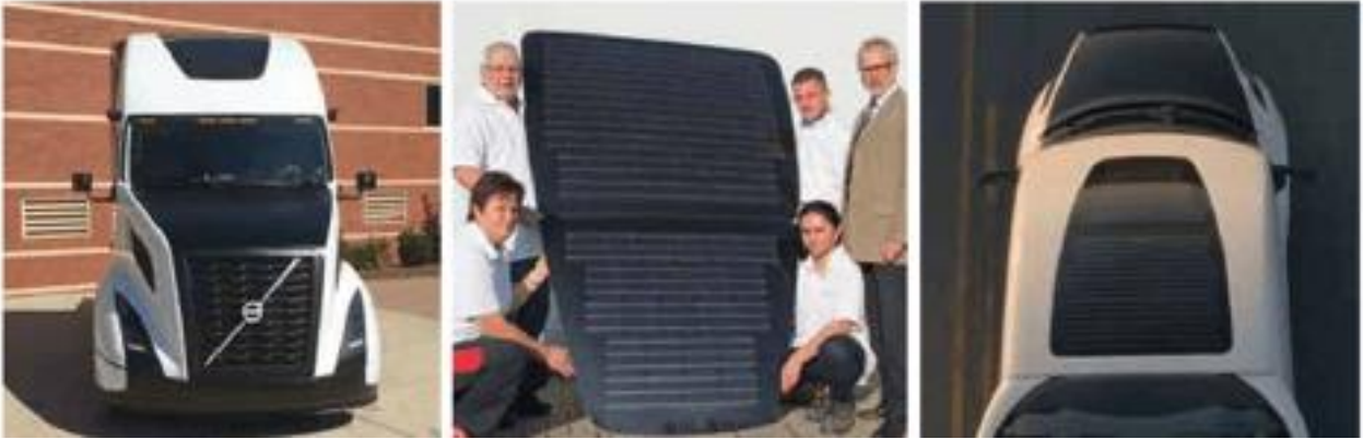
Figure 18: Spherically Curved Solar Truck Roof Modules
