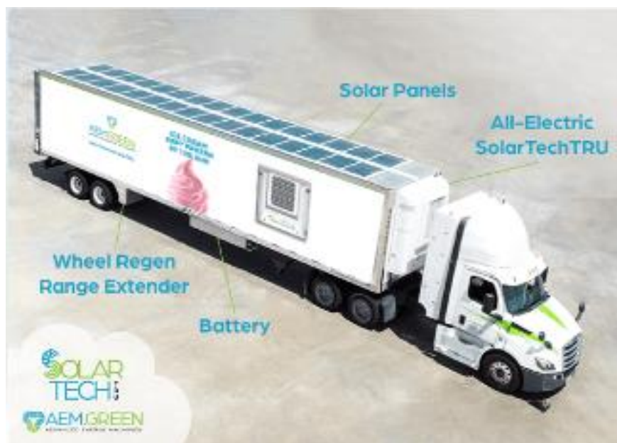
Figure 4: Volvo Electric Truck Integrated with a Reefer Trailer Equipped with a Zero-Emission SolarTechTRU
