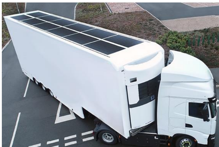
Figure 10: Merlin solar panel integrated with trucks
