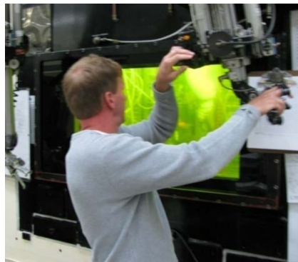
Chemical separation in hot cell REDC, ORNL, Oak Ridge
